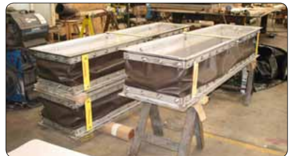
Three 81.15" L x 18.44" W x 16" High Fabric Expansion Joints for a Power Company
