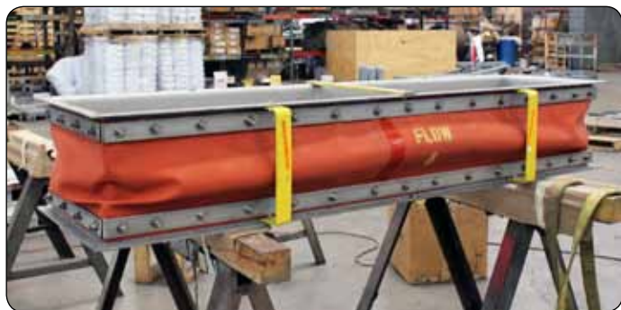
81" L x 18" W x 16" Face-to-Face Rectangular Expansion Joint Designed for High Air Circulation Flow for an Air Cooling Loop Duct in a Power Plant
