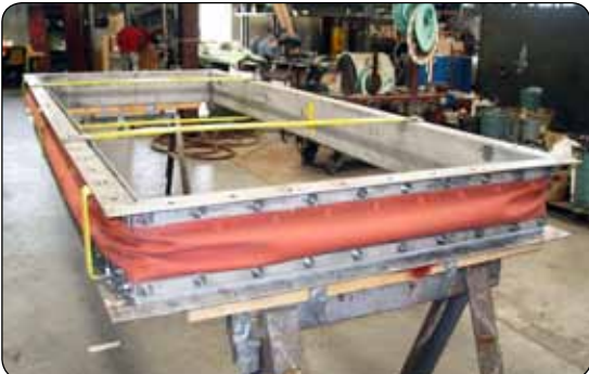
136" x 54" Fabric Expansion Joint for a Power System Company
