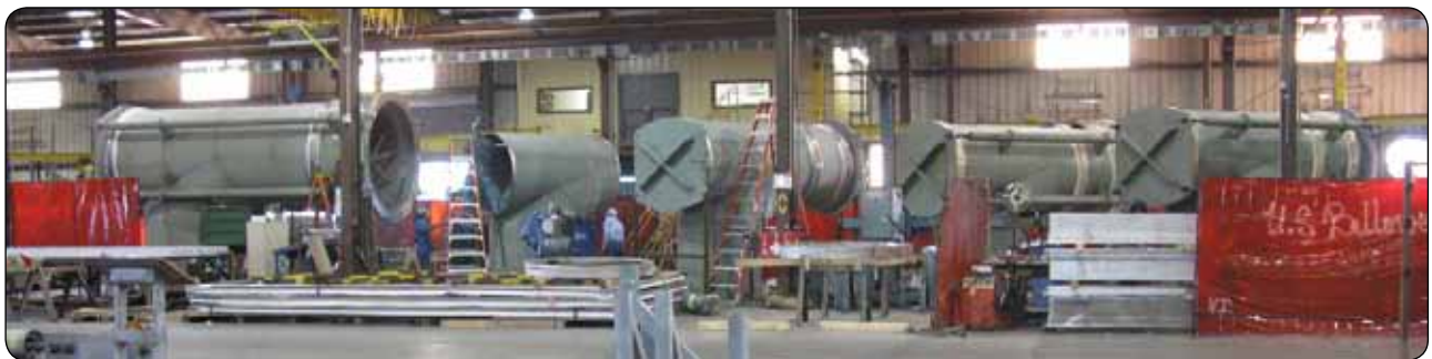
Elbow Pressure Balanced Expansion Joints being Manufactured in our U.S. Bellows Facility
