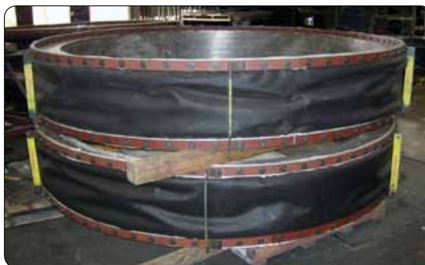
Back Up Rings Installed on Round Fabric Expansion Joints
