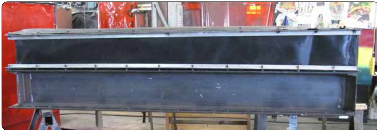
Fabric Expansion Joint for a Gas Turbine Power Plant
