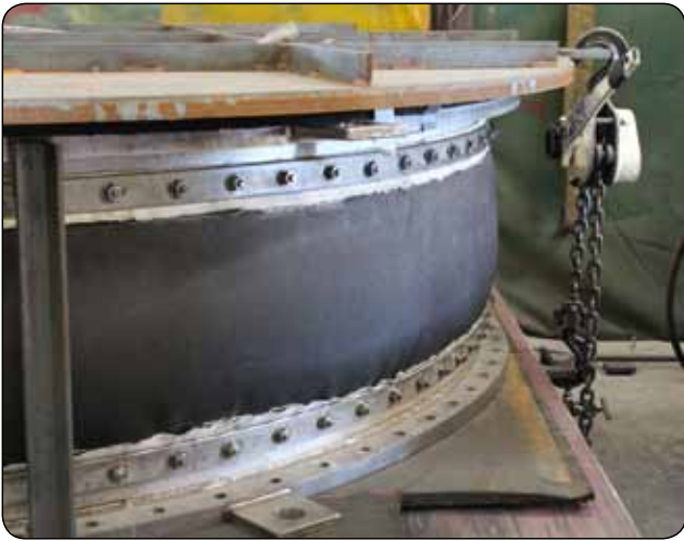
Pressure Test on a Round Fabric Expansion Joint
