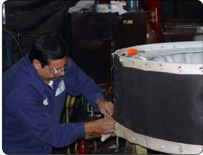
Assembling a 36" x 10" Face-to-Face Fabric Expansion Joint
